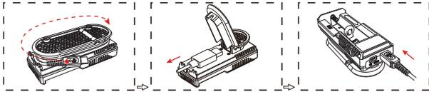
2. Inserting Battery: Insert a battery as instructed. An incorrectly inserted battery will prevent the UM10 from functioning.
